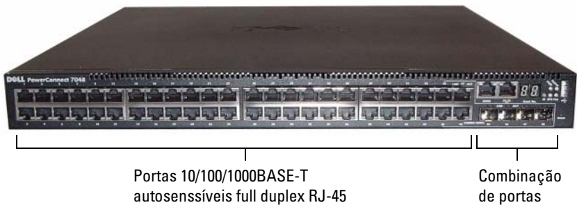
Figura 1-4. PowerConnect 7048 com 48 portas 10/100/1000BASE-T
